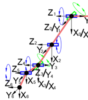
Figure 7. Graphical representation of the joint coordinate systems of the human upper limb 6 degrees of freedom kinematic model and the effector positioned on the fingertips.
