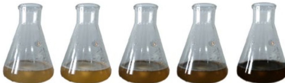
Figure 4. Colour change from yellow to brown due to reduction of \text{AgNO}_3 by aqueous extract of Cuscuta reflexa
