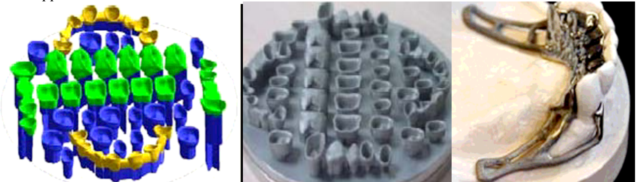
Fig.5 a) 3D Models, b) Parts manufactured, c) Dental prostheses
