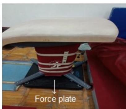
Figure 1. Set up of vault on the force plate.
